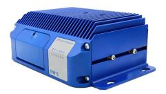
The Intelligent Vehicle Network (IVN5) is the vehicle logic unit that controls the complete Clever Devices ITS technology package on your vehicle. The brains of the vehicle, IVN5 is a rugged and powerful onboard computer specifically designed to manage your transportation applications, collecting and transmitting data, either in real-time or upon arrival in the depot.
