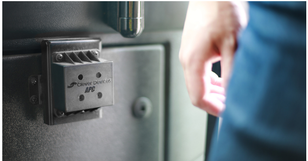
Clever Devices APC technology collects ridership data on a per-bus, per-door basis
